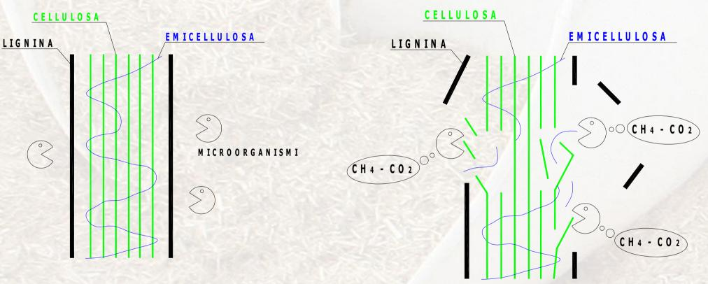
The disaggregation processes break down the shield of lignin allowing microorganisms to access the digestable carbohydrates (cellulose and hemicellulose). Furthermore, these carbohydrates are fragmented and therefore made more easily usable.
