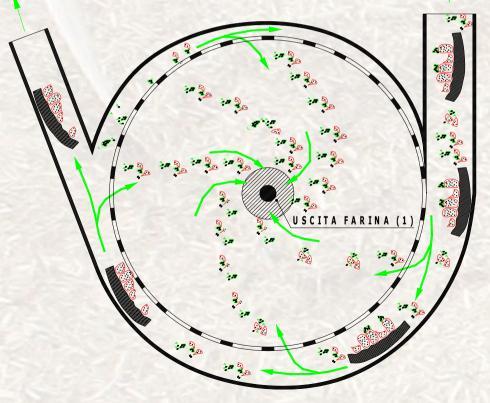
6) Fragments and air at high speed (green arrows) are introduced into the separation device and made to spin in a circular motion.
