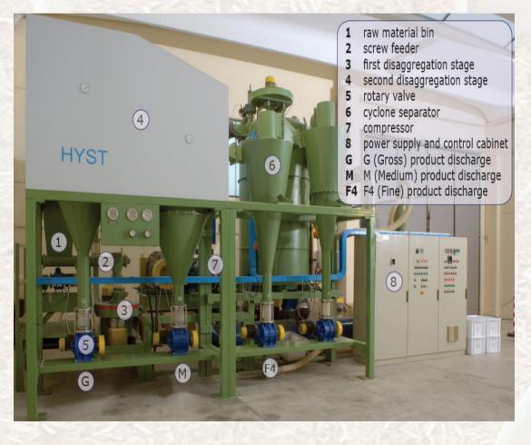
Hyst is a system designed to treat plant material through physical action.
