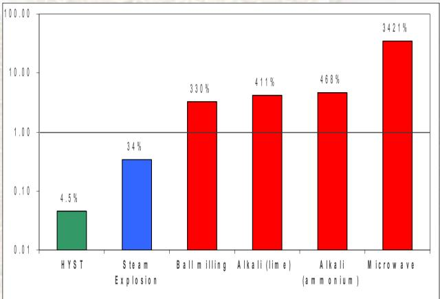
Comparing pretreatment technologies: ratio between the energy required for pretreatment (Energy Input) and that obtained from the methane produced (Energy Output).
